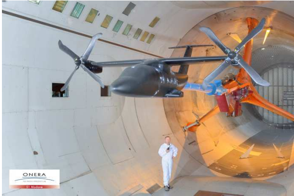
Figure 2: Aircraft configuration in the ONERA S1MA wind tunnel.
