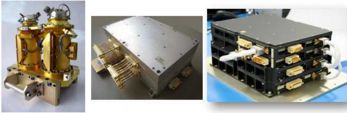
Figure 3. MICROSCOPE's Flight Model instrument. From left to right: Sensor Units, FEEU, ICU.
