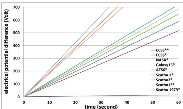
Fig. 8. Zoom of solar cells cover glasses potential difference in eclipse condition. The value of 500 V is of specific interest.
