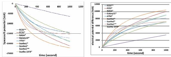
Negative spacecraft charging and inverted voltage gradient situation for cover glasses
