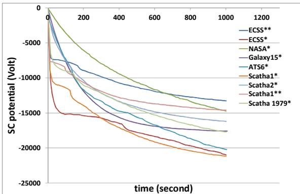
Fig. 6. Spacecraft potential versus time in Eclipse condition
