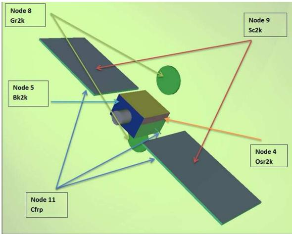
Fig. 2. Spacecraft geometry front side, with covering materials.
