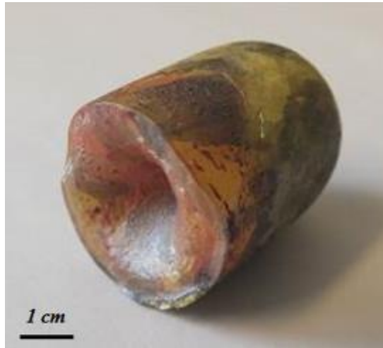
Figure 1 - AgGaGeS 4 polycrystalline ingot after the chemical synthesis
