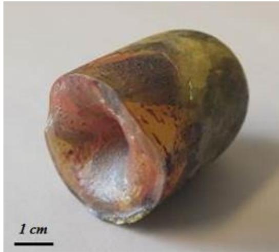
**Figure 1 - AgGaGeS<sub>4</sub> polycrystalline ingot after the chemical synthesis**
