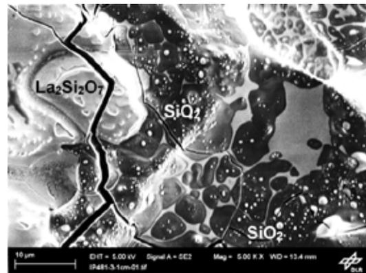
**Figure 14: LaPO<sub>4</sub>-coated fibre sample, tested at 1700°C, top view showing SiO<sub>2</sub> and La<sub>2</sub>Si<sub>2</sub>O<sub>7</sub> phases**
