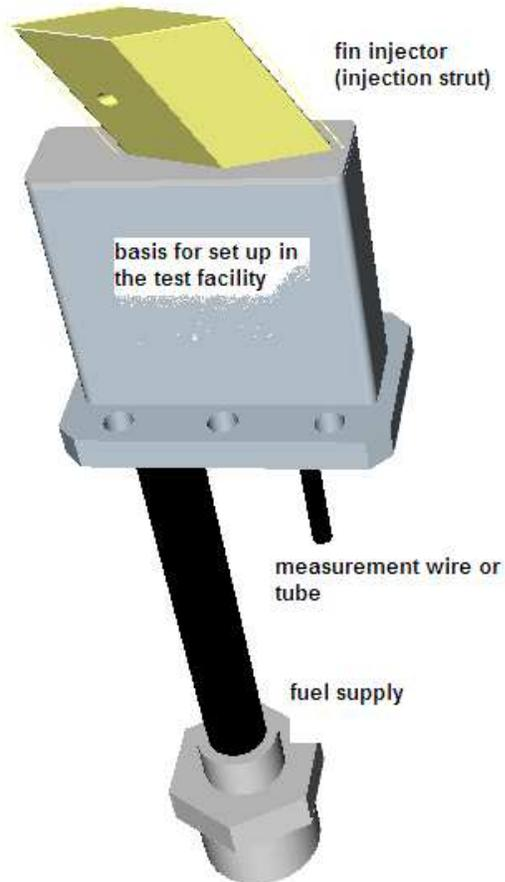
**Figure 23 : CAD view of ATLLAS2 injector on its test facility basis**
