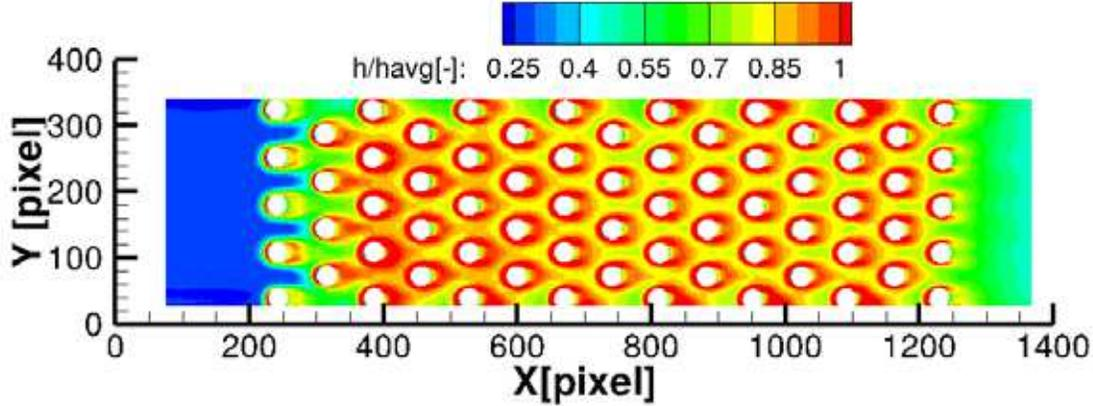
Figure 8 : Two dimensional local distribution of the normalized measured heat transfer coefficient, Case2,  $Re_{D,max}=25000$
