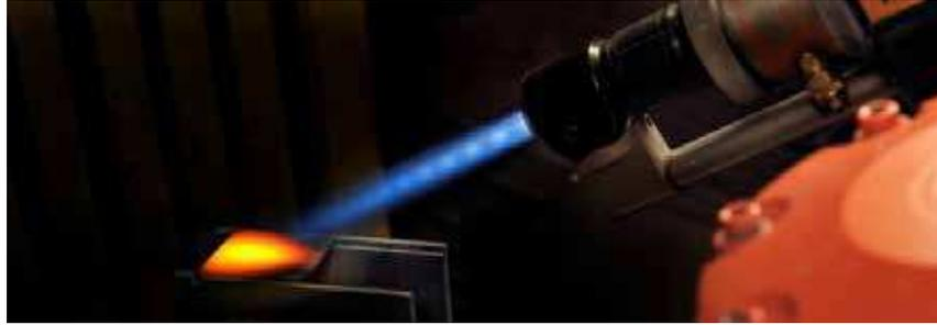
**Figure 9 : flat sample testing at ERBURIG<sup>K</sup> test facility at Airbus Group Innovations, Ottobrunn (Germany)**
