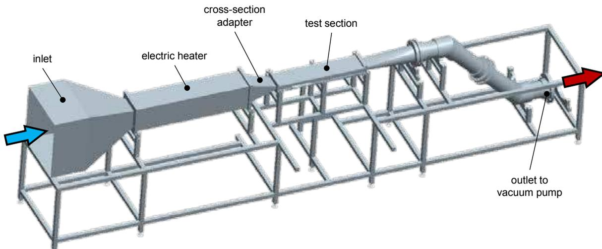
Figure 3 : Schematic view of the test facility in Stuttgart University
