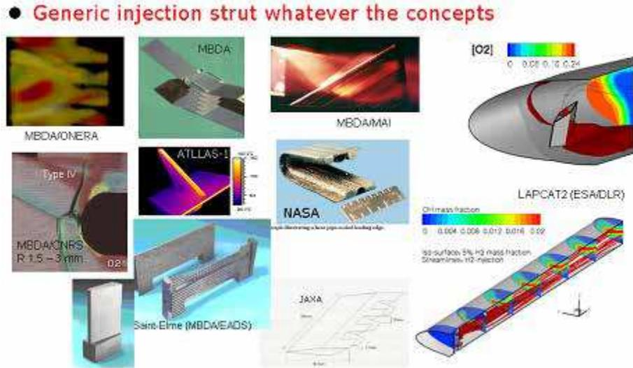
Figure 22 : examples of injection struts taken into account to define the ATLLAS2 generic fin injector
