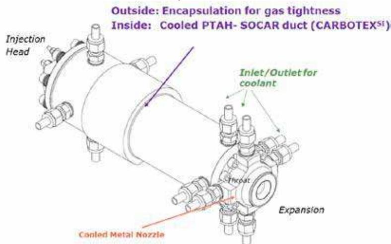
**Figure 18: cooled CMC duct for long duration testing in ERBURIG<sup>K</sup> test facility at Airbus Group Innovations in Ottobrunn, Germany**
