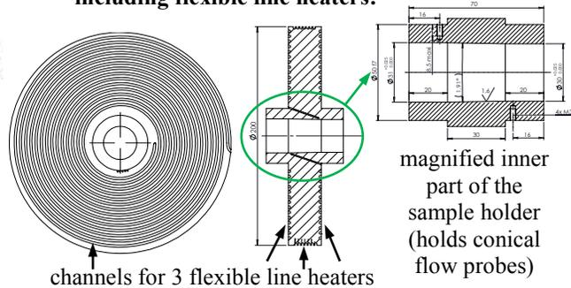
Figure 16 : Additional devices necessary for measuring the material permeability under elevated temperatures.
