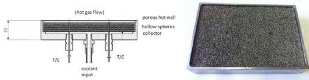
**Figure 20: HSS panel to be tested in METHYLE**
