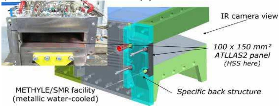
**Figure 19 : panel testing at the exit of scramjet in METHYLE test facility**
