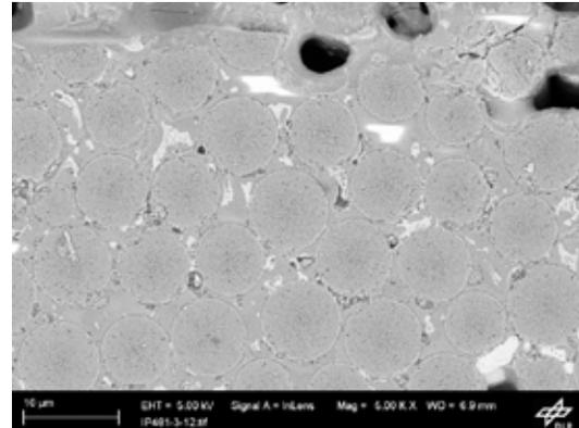
**Figure 12: LaPO<sub>4</sub>-coated fibre sample, tested at 1700°C, close to surface**
