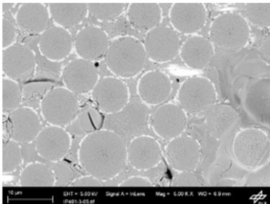
**Figure 13: LaPO<sub>4</sub>-coated fibre sample, tested at 1700°C, center of the sample**
