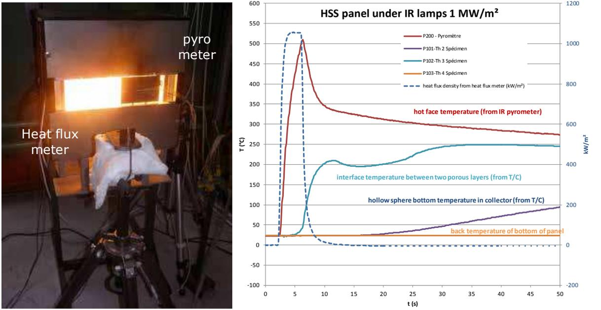
Figure 21. Infra red testing at MBDA of HSS panel
