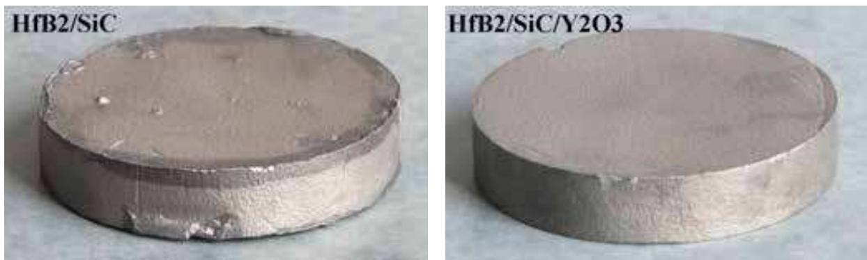
**Figure 25. UHTC materials for fin injector machining**
