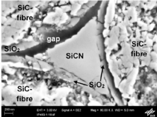
**Figure 11: PyC-coated fibre sample, tested at 1300°C, center of the sample; the PyC coating was removed due to active oxidation**
