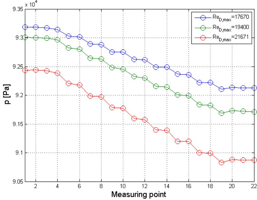
**Figure 6: Pressure distribution at the side wall of the pin fin array, Case 2**
