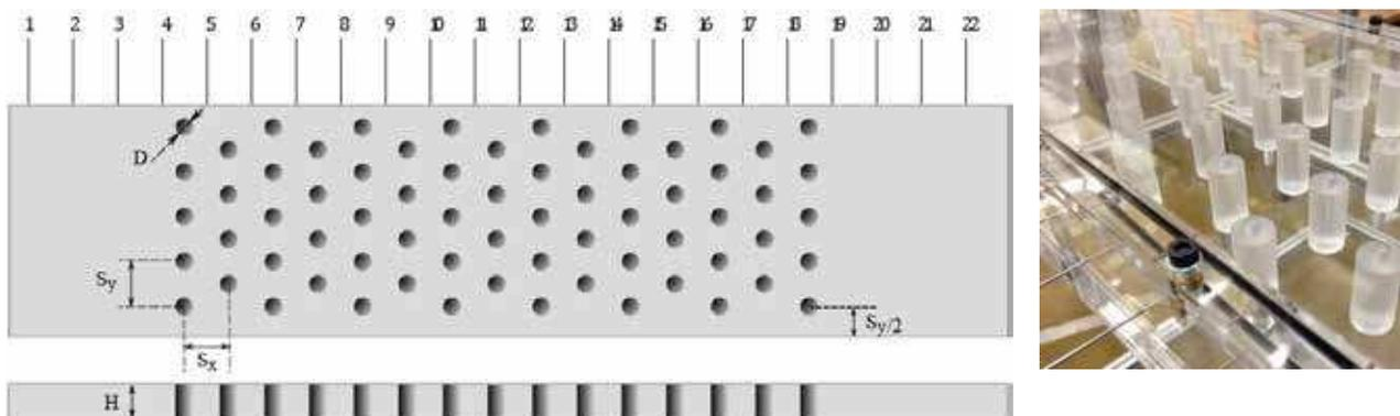
**Figure 5 : Staggered pin fin array pattern and photograph of the test section**
