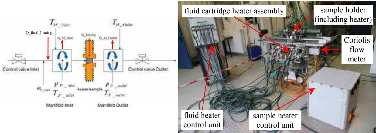
**Figure 17 : Flow scheme (left) and photograph (right) of the elevated temperature permeability measurement set-up.**
