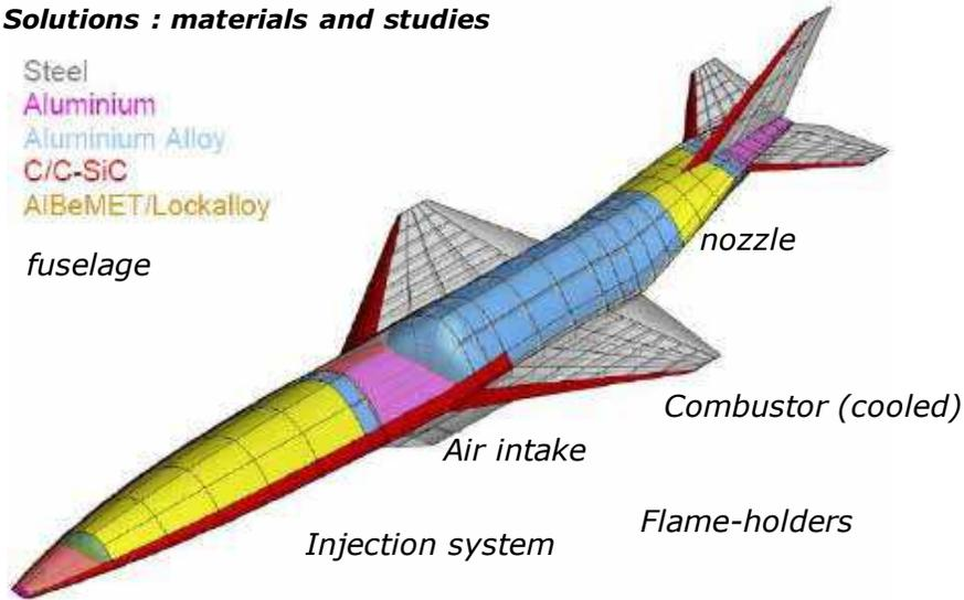
**Figure 1 : system studies as a guideline for structures to be used in different sub-systems**
