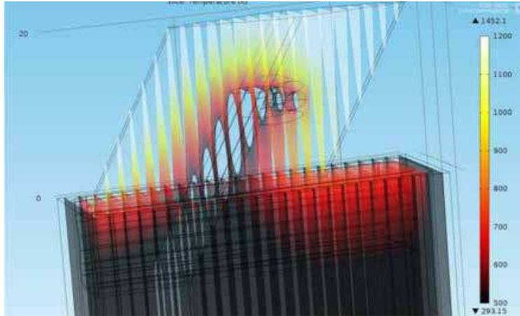
**Figure 24 : Assessment of the thermal levels (in K) in the ATLLAS2 injector (during test)**
