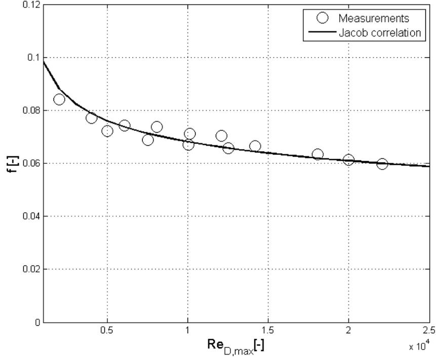
**Figure 7:** Validation of friction factor versus Jacob correlation [1] for Case 2
