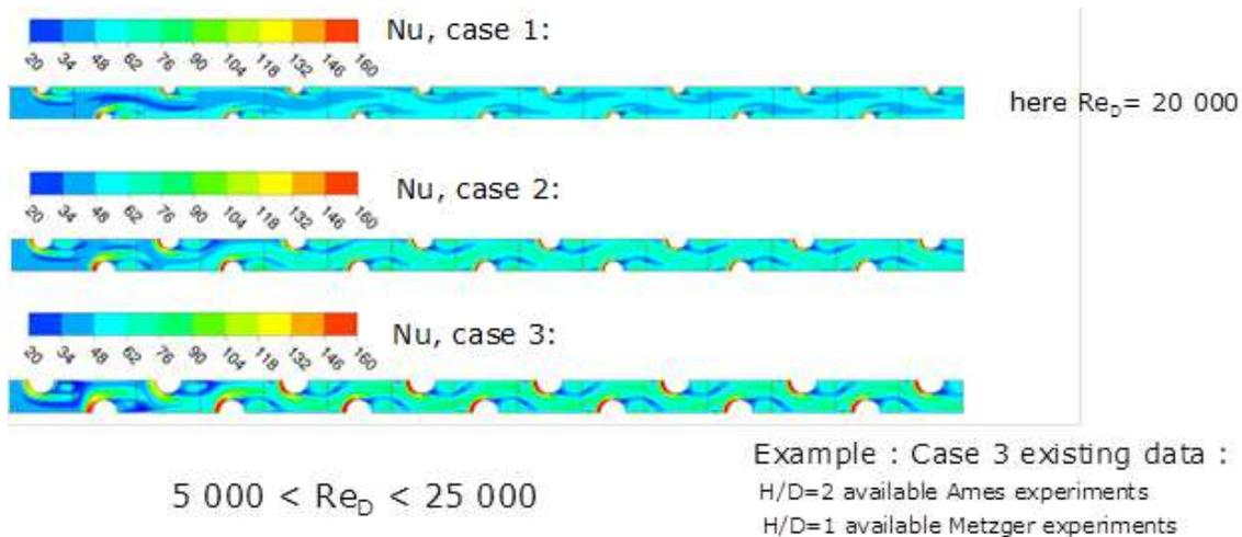
**Figure 4 : different pin fin pattern studied (here CFD results) within warm air experiment**
