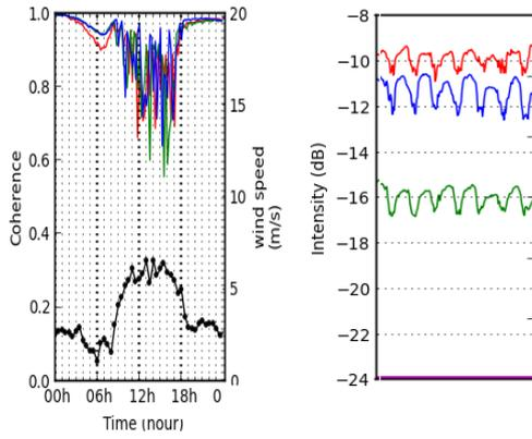
Fig. 5 : Temporal variations in the dry season. *Left* : coherence derived from HH, HV and VV scattering coefficients respectively in red, blue and green during 24 hours (reference is at 12 p.m.) The bottom curve is the wind speed. *Right* : backscattering coefficient over a period of 7 days in the dry season.
