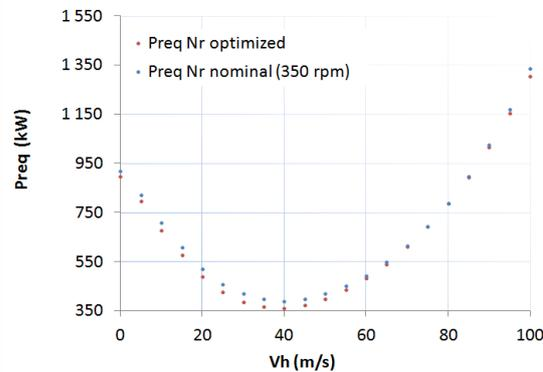
**Fig 12:** Comparison of required power in function of advancing speed for a nominal and optimized  $N_r$ .
