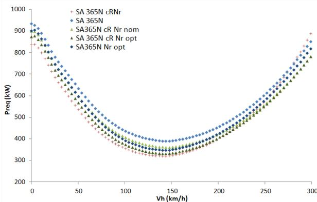
**Fig 15: Required power in hover and level flights.**
