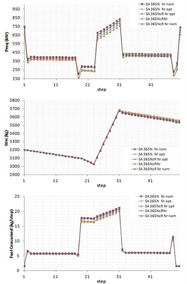
**Fig 17:** Same as figure 16 but for SAR mission. The increasing of weight at middle of the mission is due to the boarding of rescues. The rescue steps are achieved in hover and each boarding run five minutes. Thus the consumed fuel is important.
