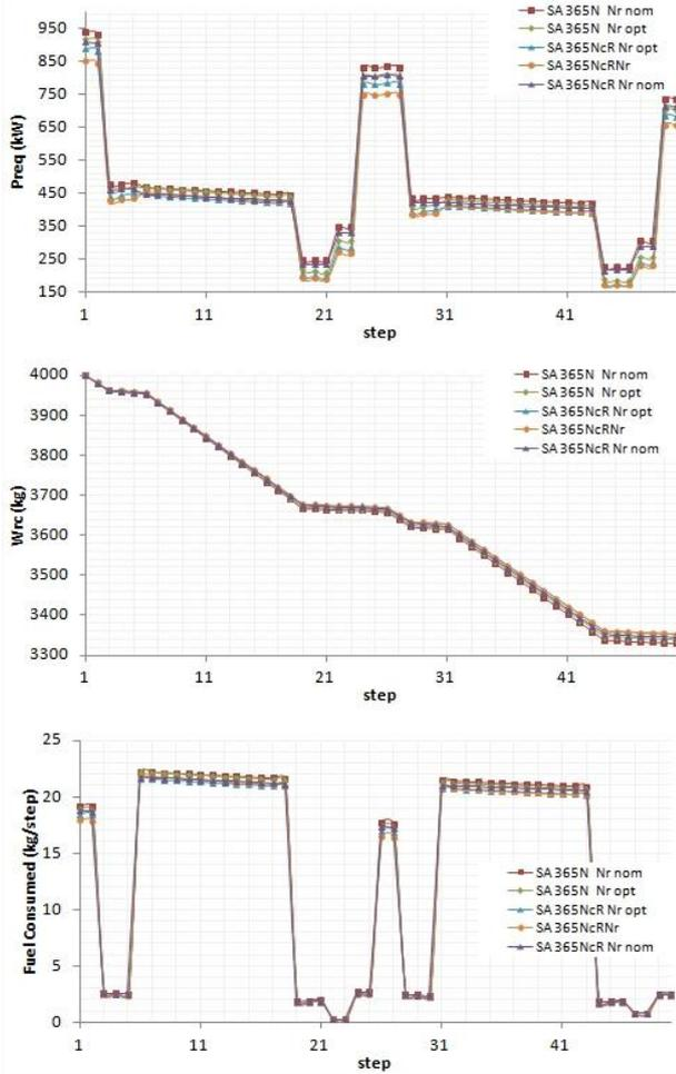
**Fig 16:** Results for offshore mission with respect to the mission steps. The first figure at top shows the variation of required power, the second one indicates the rotorcraft weight and the last at bottom presents the consumed fuel during a step. As can be seen the fuel consumed is high during the cruise although the required power is low. This is because these steps last longer in time in comparison with hover phases.
