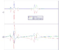
**Fig. 10 :** Example of FRFs : the real driving points (blue and green curves) and the SVDP (red curve)
