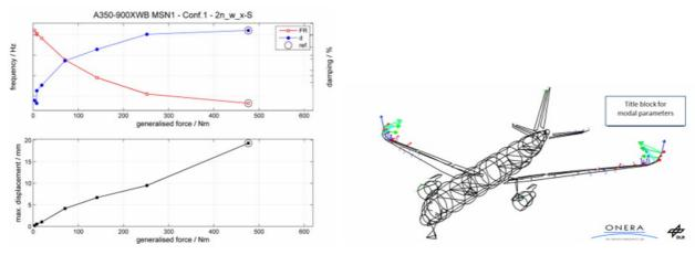
Fig. 20 : Example of linearity plot
