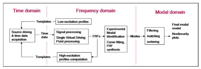
Fig. 6: Data workflow for PSM
