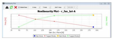
Fig. 15: Linearity plot (resonance frequency and structural damping ratio / Generalized excitation Force)
