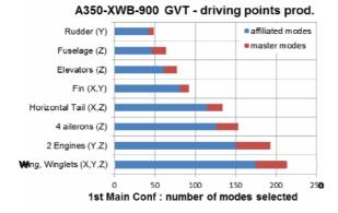
Fig. 18 : Diagram of the mode productivities of the different driving points
