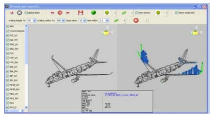
Fig. 14 : Dual mode shapes plot
