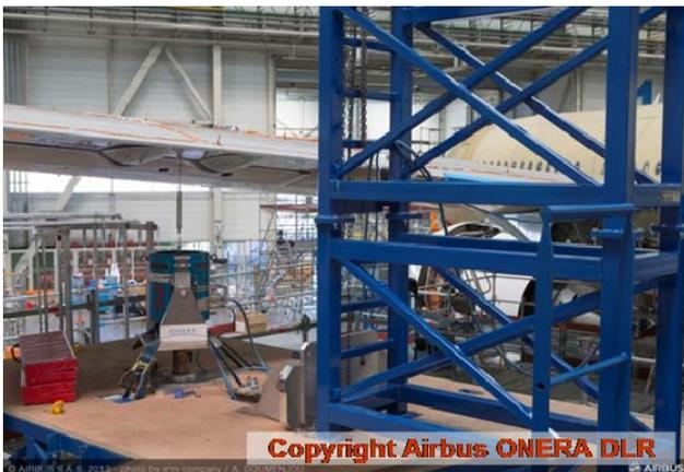
**Fig. 3 :** View of the aileron exciter (1st GVT)
