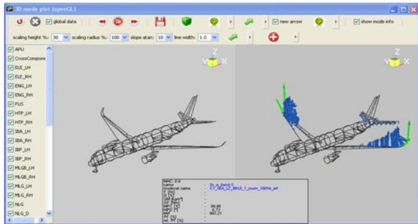
Fig. 14 : Dual mode shapes plot
