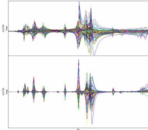
**Fig. 9 :** Example of FRFs for all accelerometers (imaginary and real parts)
