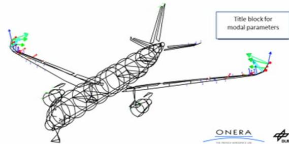
Fig. 21 : Example of mode shape plot
