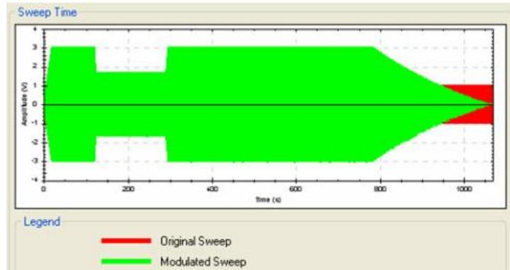
**Fig. 8 :** Example of amplitude-modulated excitation signal
