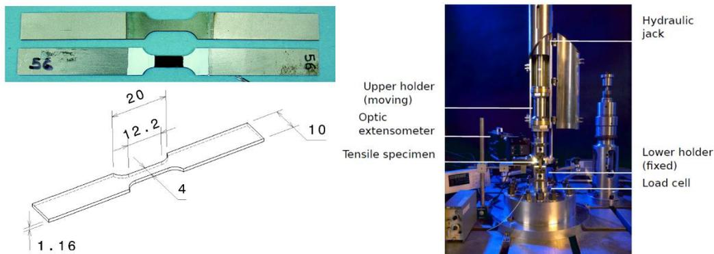
**Figure 2: Uni-axial specimen and experimental device for tensile tests at high rate of strain.**
