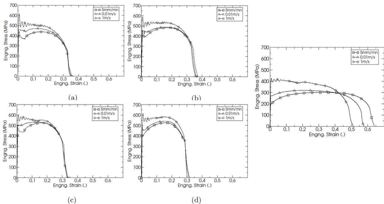
**Figure 3: Engng. Stress vs. Engng. Strain diagrams at different strain rates (0.008, 0.8 and 90s<sup>-1</sup>). (a) SC-HAZ, (b) IC-HAZ, (c) GR-HAZ, (d) GC-HAZ (right), Base Metal.**
