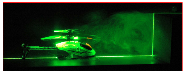
Figure 1. Flow around a small scale helicopter behind a wall in a windtunnel.
