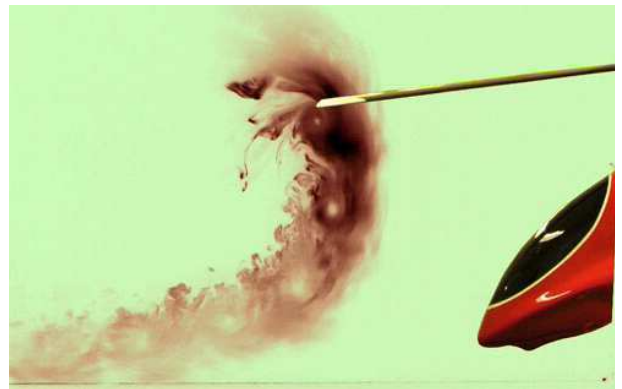
Figure 13. Photograph extracted from films in virtual colours superimposed with an image of the helicopter and a blade, side view.
