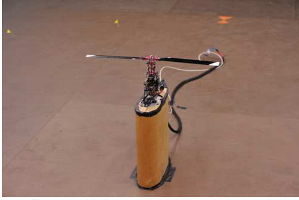
Figure 7. Helicopter in the L2 wind tunnel.
