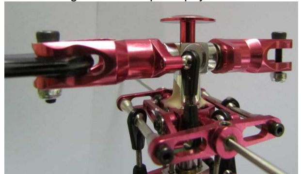
Figure 3. Rotor head mechanism, pitch commands and drag axis.
