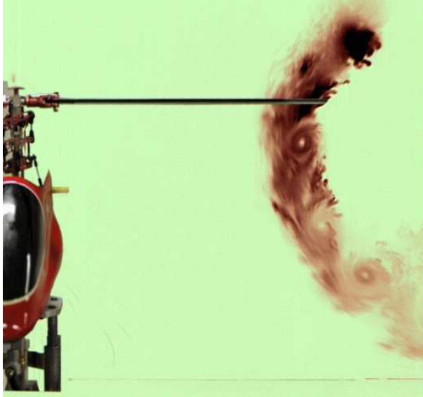
Figure 14. Front view of the shed vortices.
