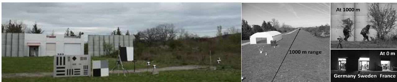
Figure 1: The 1040-m-long laser range. The targets were located from 600 to 1000 m from the sensors.
