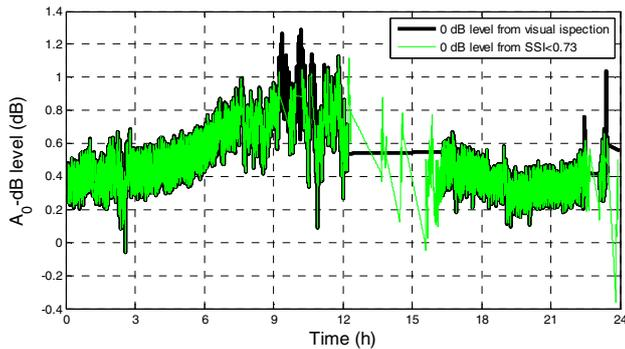
Fig. 4.  $A_0$ -dB level for the beacon measurements on December 7, 2012, using as threshold (top)  $SSI < 0.87$  and (bottom)  $SSI < 0.73$  as compared with CPA derived from visual inspection (black curve).
