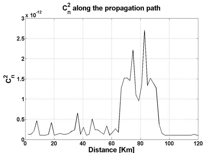
Fig. 5.  $C_n^2$  values along the propagation path for an elevation angle of  $30^\circ$ . The maximum distance of 120 km represents the horizontal distance from the center of the atmospheric volume to its edges.
