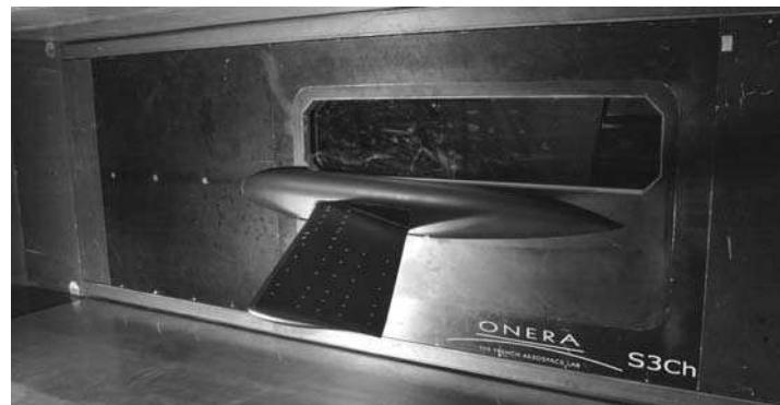
Figure 1 - Experimental set-up in the S3Ch wind tunnel.
