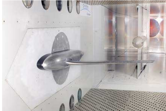
Figure 2 – AVERT model in the S2MA wind tunnel.
