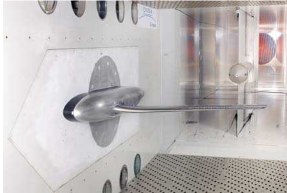
Figure 2 – AVERT model in the S2MA wind tunnel.
