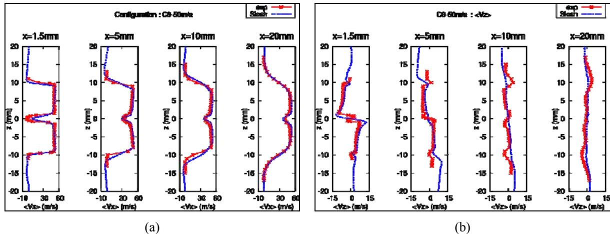
Figure 4. Vertical profiles of mean gas velocity at different distances from the injector nozzle. Comparison between 2D SLOSH simulations and experiments [3]. (a) longitudinal mean gas velocity  $\langle V_x \rangle$ . (b) vertical mean gas velocity  $\langle V_z \rangle$ .
