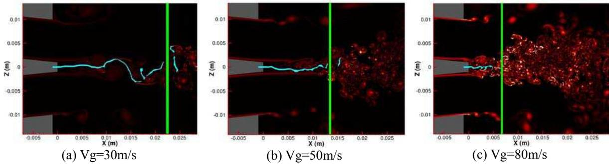
**Figure 7.** Influence of the air jet velocity on the break-up length of the liquid sheet. Cyan: snapshot of the simulated liquid sheet. Red scale: vorticity field of the gas phase. Green line: measured mean breakup length from experiments [2].
