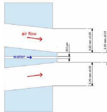
**Figure 2.** Injector layout for C9 configuration [2].
