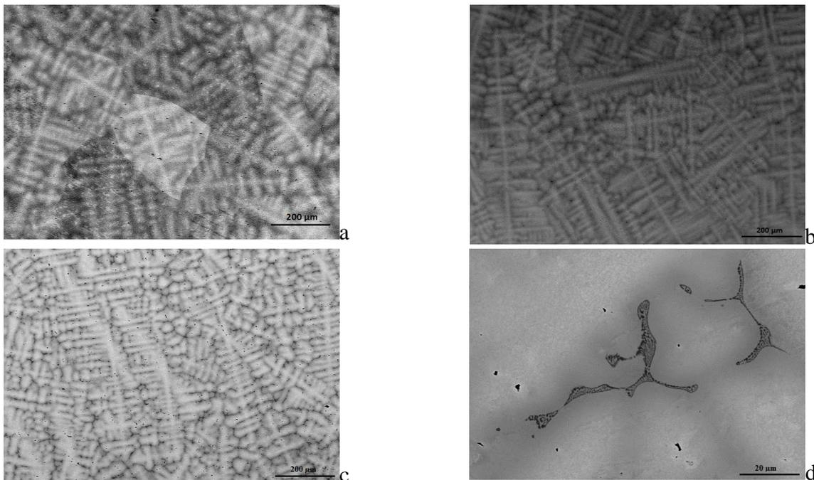
Fig. 1. Representative microstructures with BSE imaging of as-cast conditions, (a) of the M1 alloy, (b) of the M2 alloy with 1 at.% of Si, showing none presence of silicide, (c) and (d) of the M3 alloy showing a precipitation of silicide mainly located at interdendritic spaces.
