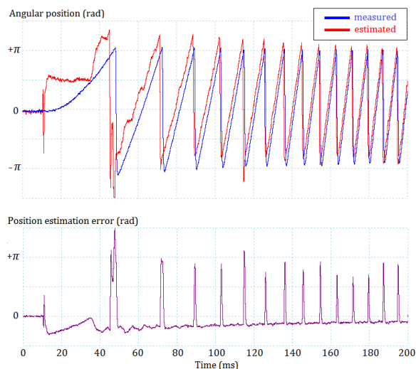
Fig. 7. Measured and estimated position for sensorless closed-loop start-up
